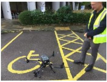
This picture shows a drone being used to survey the the civic offices, in particular the state of the concrete structure.
